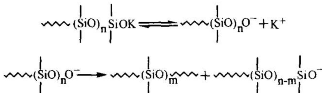
Therefore, avoiding residual monomers and catalysts helps to improve the thermal aging resistance of silicone rubber.
