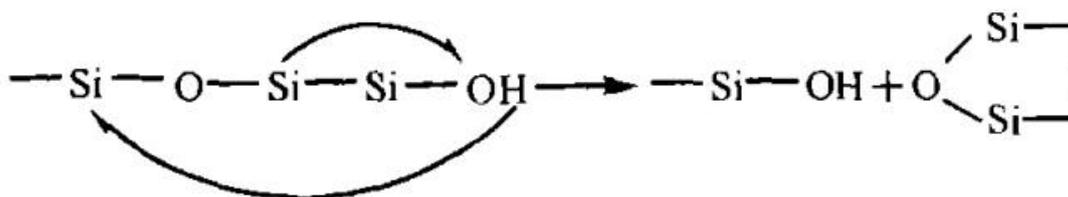
In most cases, there will be catalyst left inevitably during the silicone rubber synthesis process. Both the acidic or alkaline catalyst impact the thermal stability of silicone rubber. The vinyl silicone rubber prepared by the acidic catalyst was heated at 305 °C for 2 h in vacuum and 25% of loss weight; while the same weight loss was achieved at 256 °C prepared with basic catalyst. Examples of catalytic synthesis of silicone rubber by KOH:
