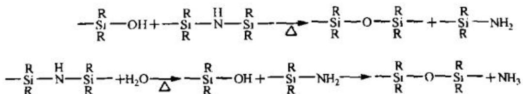
And the hydrolytic apparent activation energy of silazane, the higher the hydrolytic stability, the better thermal stability of silicone rubber will be. Commonly used silazanes are: hexamethyldisilazane, hexamethylcyclotrisilazane and so on.
